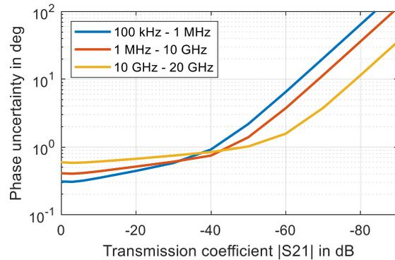
Uncertainty of transmission magnitude and transmission phase measurements for the R&S®ZNB20 in the frequency range from 100 kHz to 20 GHz; analysis conditions:  $S_{11} = S_{22} = 0$ , cal. power -10 dBm, meas. power -10 dBm
