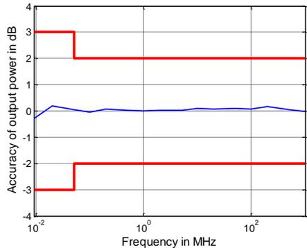
Output power accuracy in dB versus frequency for the R&S<sup>®</sup>ZNB8
