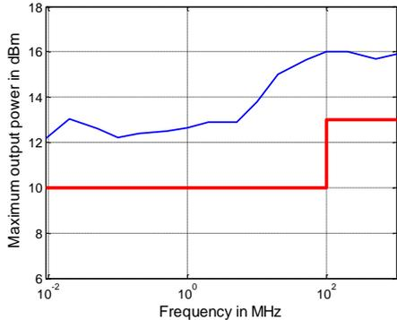
Maximum output power in dBm versus frequency for the R&S<sup>®</sup>ZNB8
