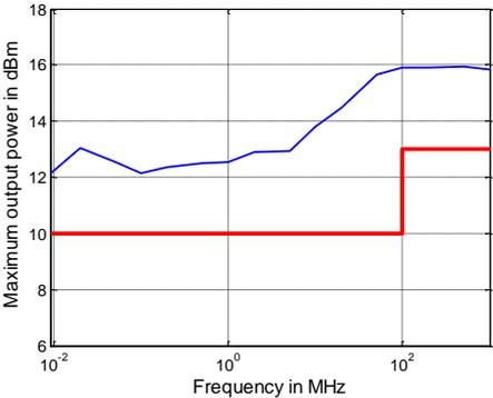
Maximum output power in dBm versus frequency for the R&S<sup>®</sup>ZNB4
