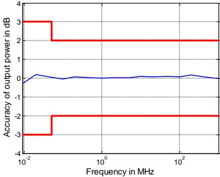
Output power accuracy in dB versus frequency for the R&S<sup>®</sup>ZNB4
