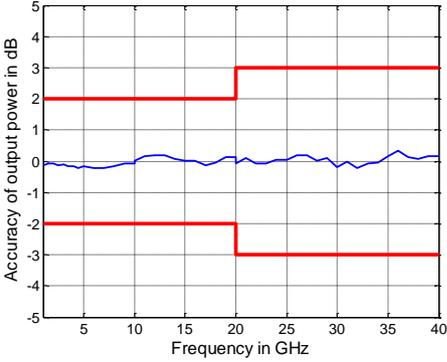
Output power accuracy in dB versus frequency for the R&S<sup>®</sup>ZNB40 model .82 and .84
