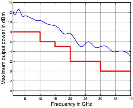
Maximum output power in dBm versus frequency for the R&S<sup>®</sup>ZNB40 model .82 and .84
