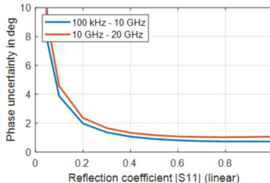
Uncertainty of reflection magnitude and reflection phase measurements for the R&S®ZNB20 in the frequency range from 100 kHz to 20 GHz; analysis conditions:  $S_{12} = S_{21} = 0$ , cal. power -10 dBm, meas. power -10 dBm
